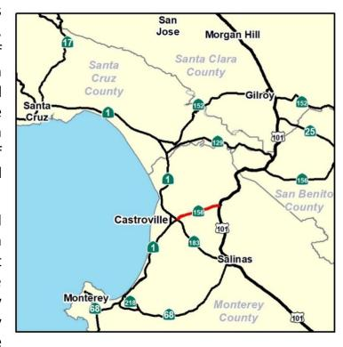
addressed. The State Route 156 West Corridor Improvement Project will construct a new four-lane expressway parallel to the existing route, with new interchanges constructed at Castroville Boulevard and at U.S. 101. The current two-lane highway will be converted into a frontage road that will provide safer community access, including for active transportation modes. The result will be improved safety and traffic flow in the area.
