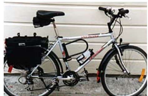
Typical commuting bike, complete with essentials such as fenders, bell, locks, kickstand and lights.
