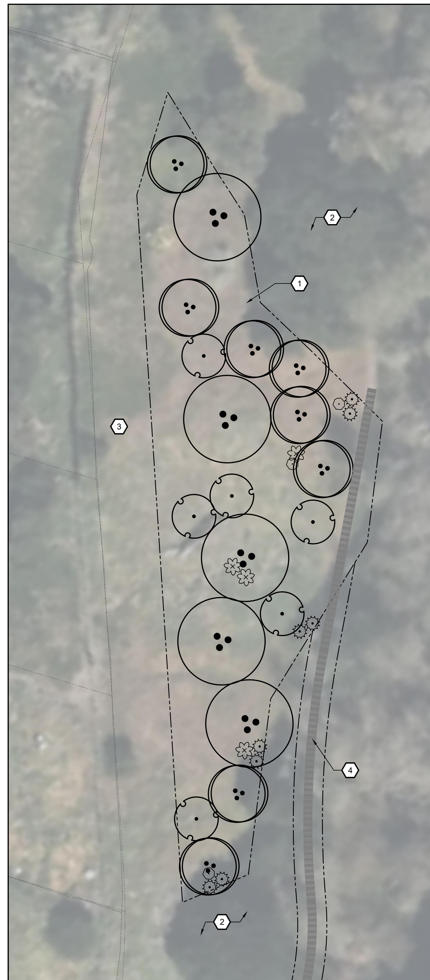
RIPARIAN MITIGATION AREA A TOTAL AREA: 12,243 SF TOTAL # OF TREE: 19 TOTAL # OF SHRUBS: 15
