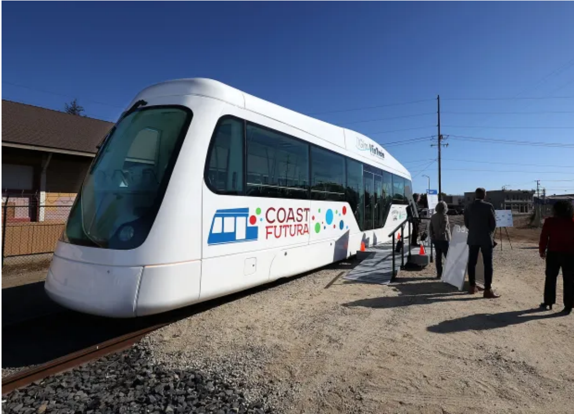
The Coast Futura demonstration rail vehicle seen Friday in Watsonville is a battery-dominant hydrogen fuel cell hybrids manufactured by California-based TIG/m. (Shmuel Thaler/Santa Cruz Sentinel)
