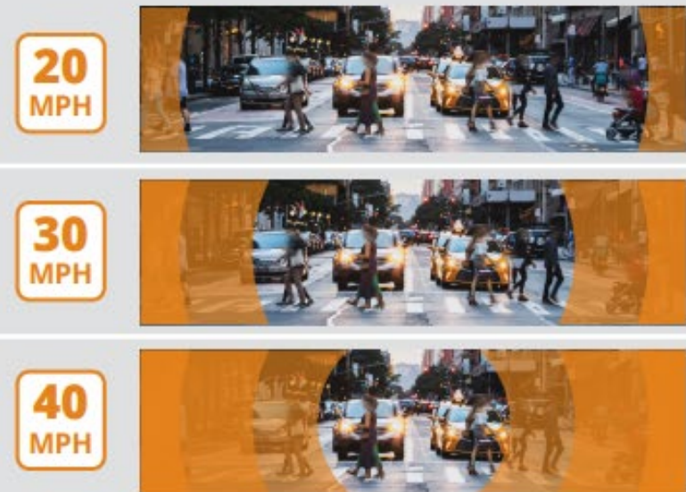
FIGURE 6. EFFECT OF SPEED ON A DRIVER'S FIELD OF VISION
